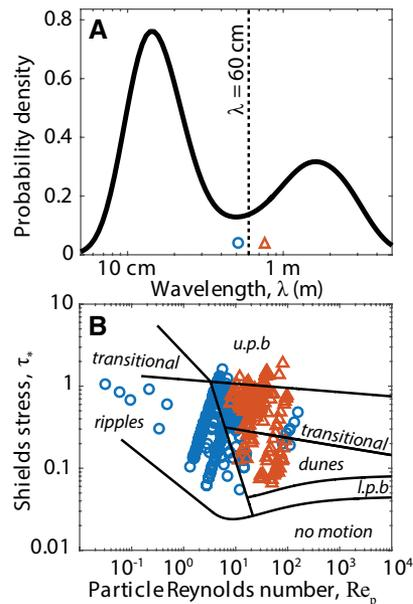
**Figure 1. A:** Probability density of bedform wavelength (Table DR1; see footnote 1), and the 60 cm threshold of Ashley (1990) (vertical line). **B:** Bedform stability diagram (from Southard and Boguchwal, 1990a; van den Berg and van Gelder, 2009; as synthesized by Lamb et al., 2012) with ripples (blue circle) and dunes (red triangle) discriminated by the 60 cm threshold. Abbreviations: l.p.b—lower plane bed regime; u.p.b—upper plane bed regime.
